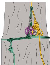
multiANCHOR used as basal anchor
