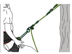
Single configuration, together with the Thimble Loop
