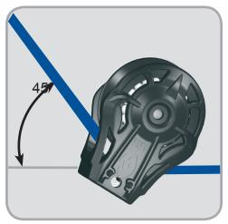
For a 45° angle: The load factor will be 75%. A load of 100 Kg on the line will represent a load of 75 Kg on the block.
