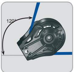
For a 120° angle: The load factor will be 180%. A load of 100 Kg on the line will represent a load of 180 Kg on the block.
