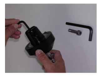
We recommend to use the supplied Loctite glue to hold definitively the snapshackle screw in position once you have found the final orientation.
