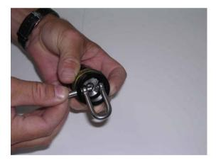
The horizontal shackle pins and the shackle can now be removed. Insert the head of the sail/halyard into the shackle, put the pin back in place and then put the rubber circlips back onto the circular groove.
