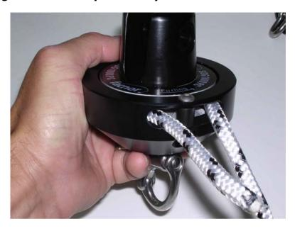
We advise you use a furling line of **8 mm diameter** for the **SDG 1000 PC** and **10mm diameter** for the **SDG 2000 PC**. Place the end of the furling line into one of the holes and turn the drum mechanism. The drum will grip the furling line. A small screwdriver may be used to help the line out of the exit hole if necessary.
