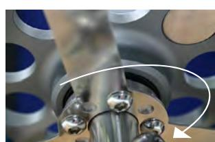
**9 & 10** - The stainless steel guide can be adjusted in order to correctly orientate the furling line according to the chain plate attachment (see installation instructions).
