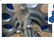
Introduce the 4 screws into the previously marked holes and quickly tighten. Remove any residual alue.
